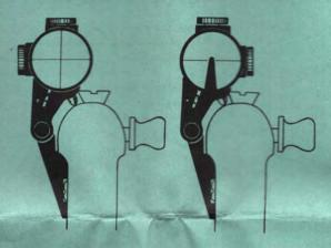
1. The base mount is shaped to fit receiver as shown above. A scope having a post reticule must be positioned forward for enough so that empty case, when ejecting, will clear windage adjusting screw. Cross hair reticule permits mounting closer to eye, since scope may be rotated ¼ turn, as shown, so shells will clear scope when ejected.
