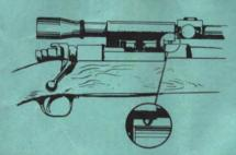
position. This stop pin may be ground shorter if necessary to bring scope to lowest possible position. (Take care that bolt will clear scope and function properly).
