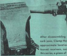
After disassembling rifle, clamp barrel in vise between cork jaws. Clamp the jig loosely in place on action in the approximate location for the base mount. On some contoured receivers, such as the remodeled Enfield used in this series, a piece of thin paper under the clamp will keep jig from slipping out of location on contoured receiver
